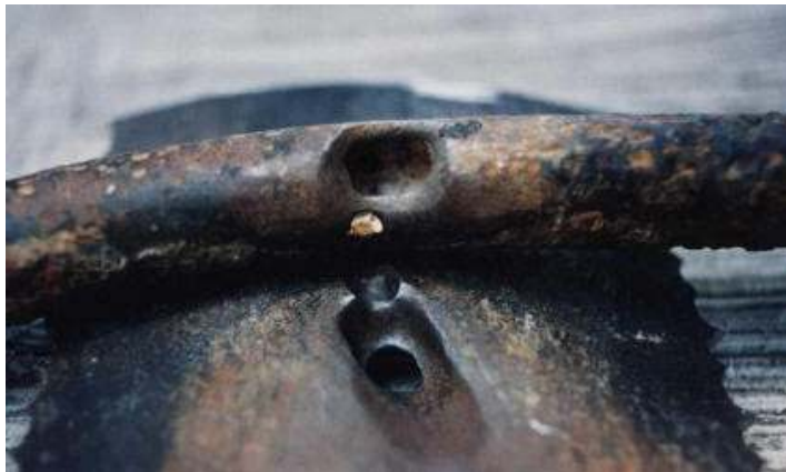
Pitting corrosion of Ti in CH 3 OH-LiCl solutions
